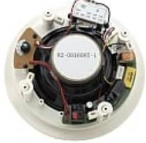
The Galil 6-CO is a pair of two-way open-back 8Ω speakers designed for mounting in the ceiling. The speakers feature a multi-tap power transformer for selecting direct 8Ω (bypassing the transformer) or 70V/100V power settings suitable for array installation
